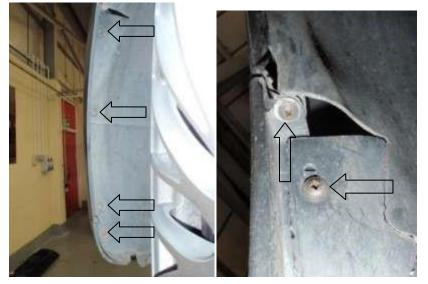
6. Remove 8x T20 Torx screws from the under tray. Completely remove the under tray from the vehicle.
