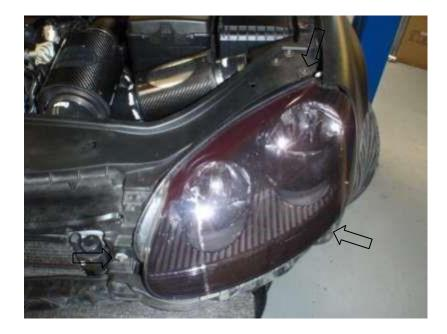
14. Un-clip the fog light wiring that runs along the bottom edge at the front of the car. Also unclip wiring from right-hand side.
