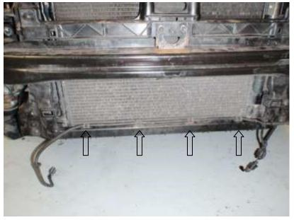
15. Disconnect the sensor located near the radiator in the top left-hand corner.
