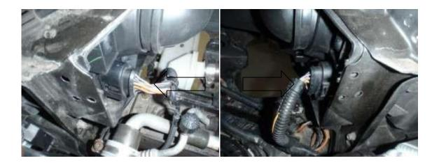
12. Unscrew 2x T20 on the headlight support. Remove the headlight support from the vehicle. The headlight supports are handed (Right & Left) so may need to be marked to help with reassembly.
