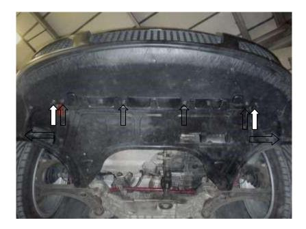
7. Pull forward on each side of the bumper to release it from its mounts underneath both lights. Carefully pull the bumper away from the car.
