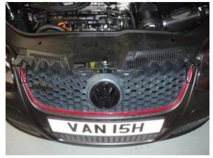
3. Remove the 2x T20 Torx screw hidden below the number plate surround. Pull the grill upward to release it form the car.
