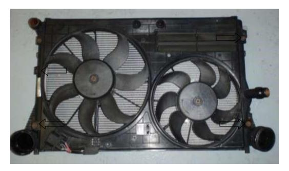
28. Carefully position your new Forge intercooler against the radiator and bolt together using 4x M6 X 12mm and 4x M6 washers supplied.
