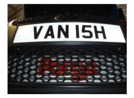
4. Remove 2x T30 Torx screws on the top edge of the bumper cover.
