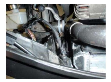
16. Disconnect the bonnet pull cable. The junction box is above the left-hand headlight. Open the junction box and disconnect the cable. <u>Ensure this is reattached correctly when</u> <u>reassembling the vehicle otherwise you will be unable to reopen the bonnet.</u>
